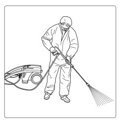
**13.** Switch on high-pressure cleaner with opened spray gun. Bleed appliance: Gun has to be opened and closed several times. Start cleaning task.
