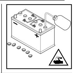
The W345B & W355B machines use two 12 volt batteries, the W365B & W375B machines use four 6 volt batteries.
