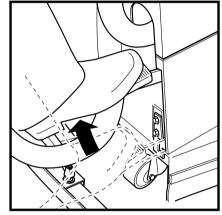
Press the brush motor on/off push button to engage the brushes. Press the brush pedal down and latch it into its lower position, press the brush push button again to stop the motors.
