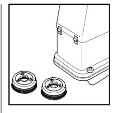
Move the machine forward until the brushes are pushed along the floor. Release the brush lift/ lower pedal and allow it to settle at its highest point. Rock the machine forward and back about 50mm (2") to settle the drive plates into the brush centers.
