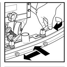
Push the coiled end of the squeegee hose fully home onto the tubular spigot in the centre of the squeegee.
