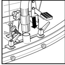
Push the straight end of the squeegee hose onto the tank inlet pipe which protrudes through a slot in the lower rear panel.
