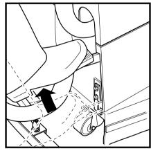
Drive the machine forward by holding the hand-grips. And turning the thumb wheels.
