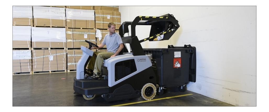
If the machine has been used until flashes the battery level indicator on the display machine, a full recharge of the batteries (10-12 hours) will be required. Failure to carry out this this procedure may cause damage to the batteries. Charging the batteries after every use is recommended.
