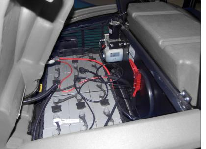
2. For the battery model, check the battery compartment is clean.
