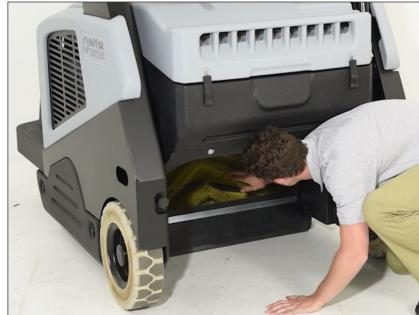
3. Check that the main broom can freely rotate and is free from ropes or debris.
