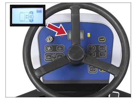
1. Check the diesel fuel tank level/LPG bottle/ battery level.
