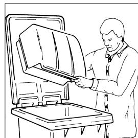
Empty the dirt collecting tank at regular intervals. The machine will no longer sweep when the tank is full.
